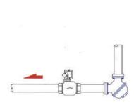
It's easy to cause water hammer effect when the gate closes fast. To set up arrester at the first corner away from the fast-shut-down valve can absorb and prevent the water hammer effect directly and eliminate the noise.
