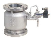
Solenoid control valve is a kind of isolation valve, which can substitute traditional gate valves, ball valves and butterfly valves. The gate functioning is easily controlled by electrical power. The valve can be installed in fire control facility, water supply, or distant location where it's difficult to control the gate opening. The controller is directly fixed and can be easily installed on piping site. Interchangeable between manual and solenoid control.
