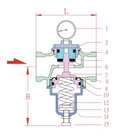
Pressure Adjusting Range :  $1 \sim 6 \text{ kgf/cm}^2$ (  $1 \text{ kgf/cm}^2 = 14.2 \text{ psi}$ )  $4 \sim 10 \text{ kgf/cm}^2$  $8 \sim 13 \text{ kgf/cm}^2$
