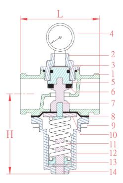
$CV = \frac{Q}{\sqrt{\triangle P/S}}$  Q = GPM (gallon/min )  $\triangle P = P1 - P2 \text{ (p.s.i)}$  P1 = Inlet absolute pressure P2 = Outlet absolute pressure S = Fluid Density (Water=1) 1 gallon=3.785 liter
