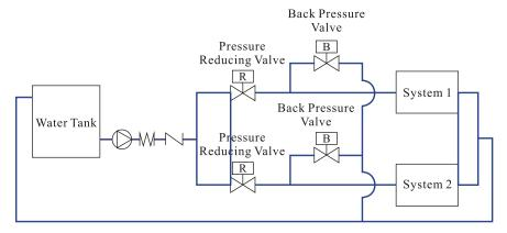
⊚In different pressure systems of processing pipelines, installing back pressure valve can maintain required pressure of the systems and ensure safe ues of equipments after pressure reducing valve reduces pressure.
