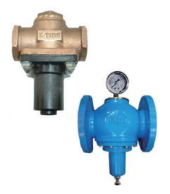
▶ Pressure Relief Valve is a safety device for pipes and it is normally closed. When pressure increases to setting value, pressure relief valve rapidly releases the over high pressure. When pressure returns to safety value, pressure relief valve will automatically close to ensure the safety of equipment.
