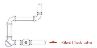
When the fluid flows through the serial corner, the change of flow speed and direction and friction effect will cause unstable pressure wave, which will lead to vibration and noise. To set up arrester and silent check valve can eliminate the pressure wave.
