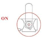
When the handle is rotated upward, pressure reducing valve set becomes pressure reducing open state.
